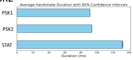
Performance metrics (time, memory, energy) are measured using the nRF52840 development board, the Saleae Logic Analyzer and Otii Arc (power profiler device)
